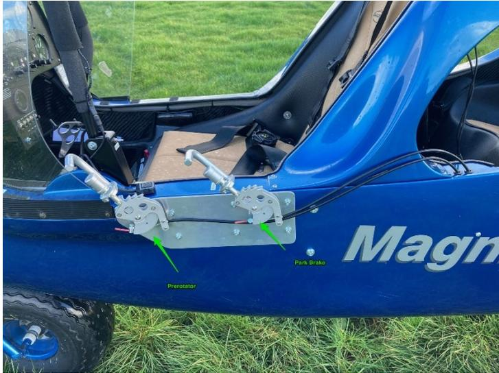
RPA the first Magni in NZ to be converted (five years ago ) onto bush tyres & nosewheel suspension assembly. It has now been converted to hand controls for its new owner in Christchurch. Test flying this month & training to begin in October.
