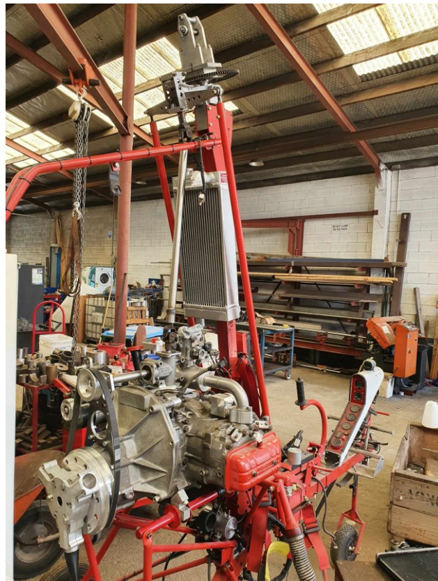
New radiator, and pre rotator under construction
